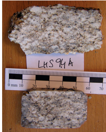
Fig. 32. The character of medium-coarse-grained, more leucocratic types of granodiorite rocks with irregular spatially and size-distributed biotite.
