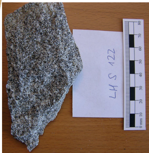
Fig. 42. Fine-grained omnidirectional, grey biotite-rich microgranodiorite-microtonalite, as one part of the biotite granodiorite-tonalite body (sample LHS-122 – Krstenica valley).
