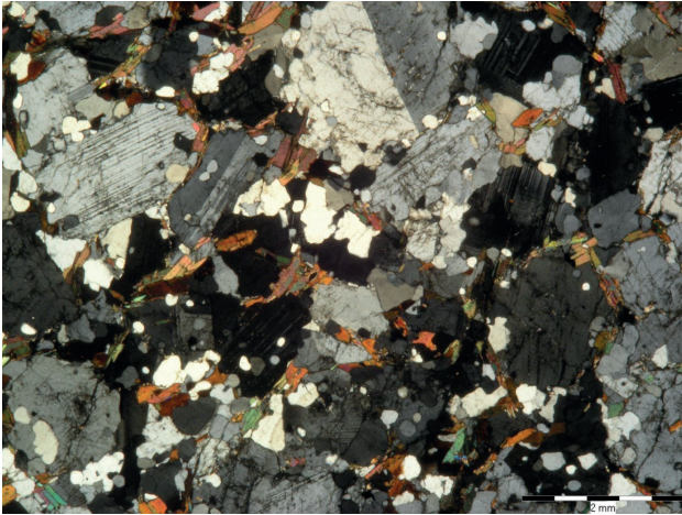
Fig. 43. Granite sample LHS-94B. Hypidomorphic plagioclases are zonal, crystallizing first in crystallization succession. Only rarely in their final phase of crystallization the interstitial K-feldspar crystallized. NX.
