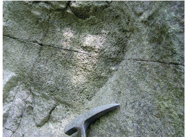
Fig. 41. Biotitic granodiorites – tonalites – mixing of two types – block of more mafic part rich in plagioclase and the biotite rich part (above hammer) in more quartzy coarser-grained rock.
