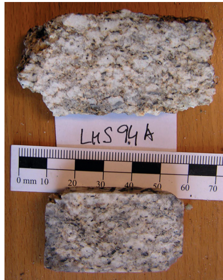
Fig. 32. The character of medium-coarse-grained, more leucocratic types of granodiorite rocks with irregular spatially and size-distributed biotite.
