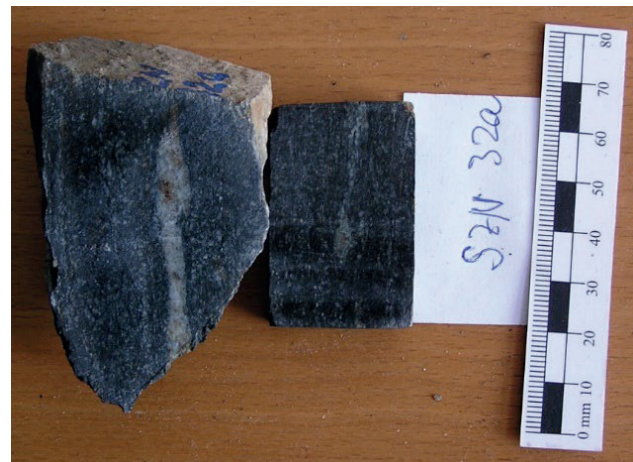
Fig. 5. Dark-grey amphibolite rock with thin light-grey interbed of diopside pyroxene (area of Železná dolina valley, sample SZN-32a).
