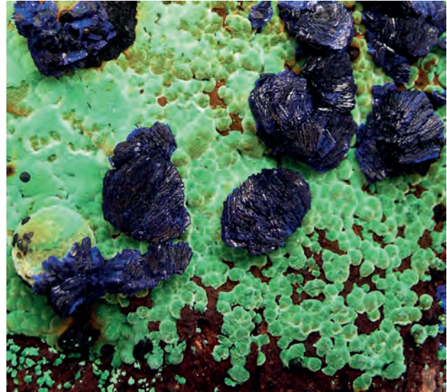
Fig. 2.7 Aggregates of azurite composed of dark blue, glossy, table-shaped crystals grown on malachite. The slit width is 2.9 cm. The size of the largest aggregate of azure at the centre of the image is 8 mm. Photo: D. Ozdín
